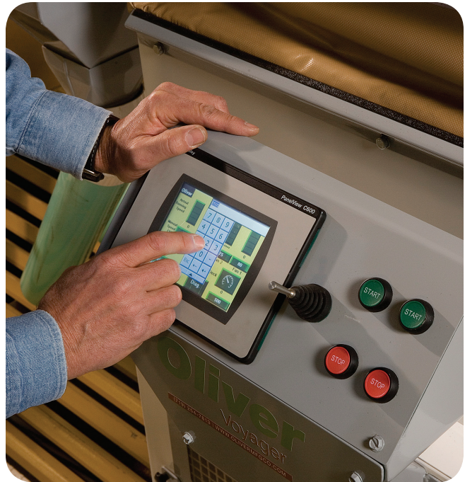
Allen-Bradley PanelView Component C600 touch-screen human machine interfaces allow operators to program product recipes and automatically return to previously defined machine settings.
