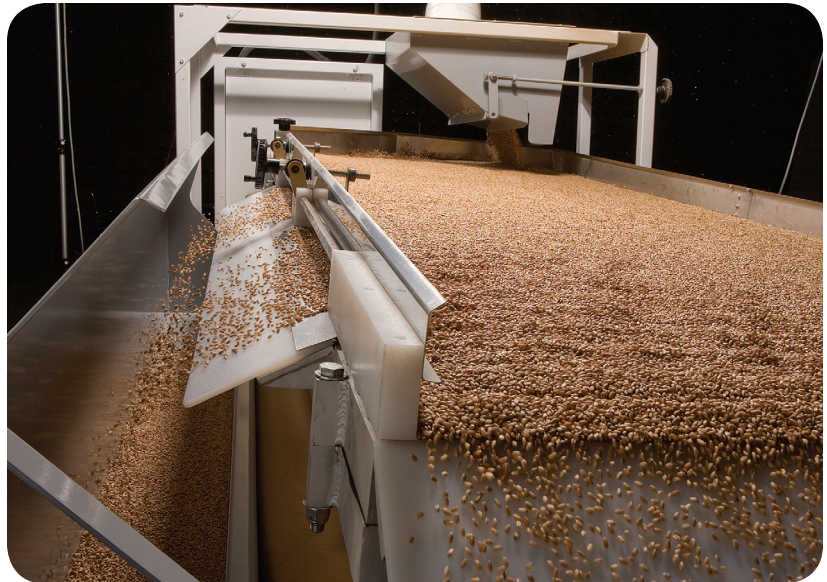
Oliver Manufacturing delivers gravity separator machines to help improve the quality of raw materials and finished food products by sorting and removing contaminants.
