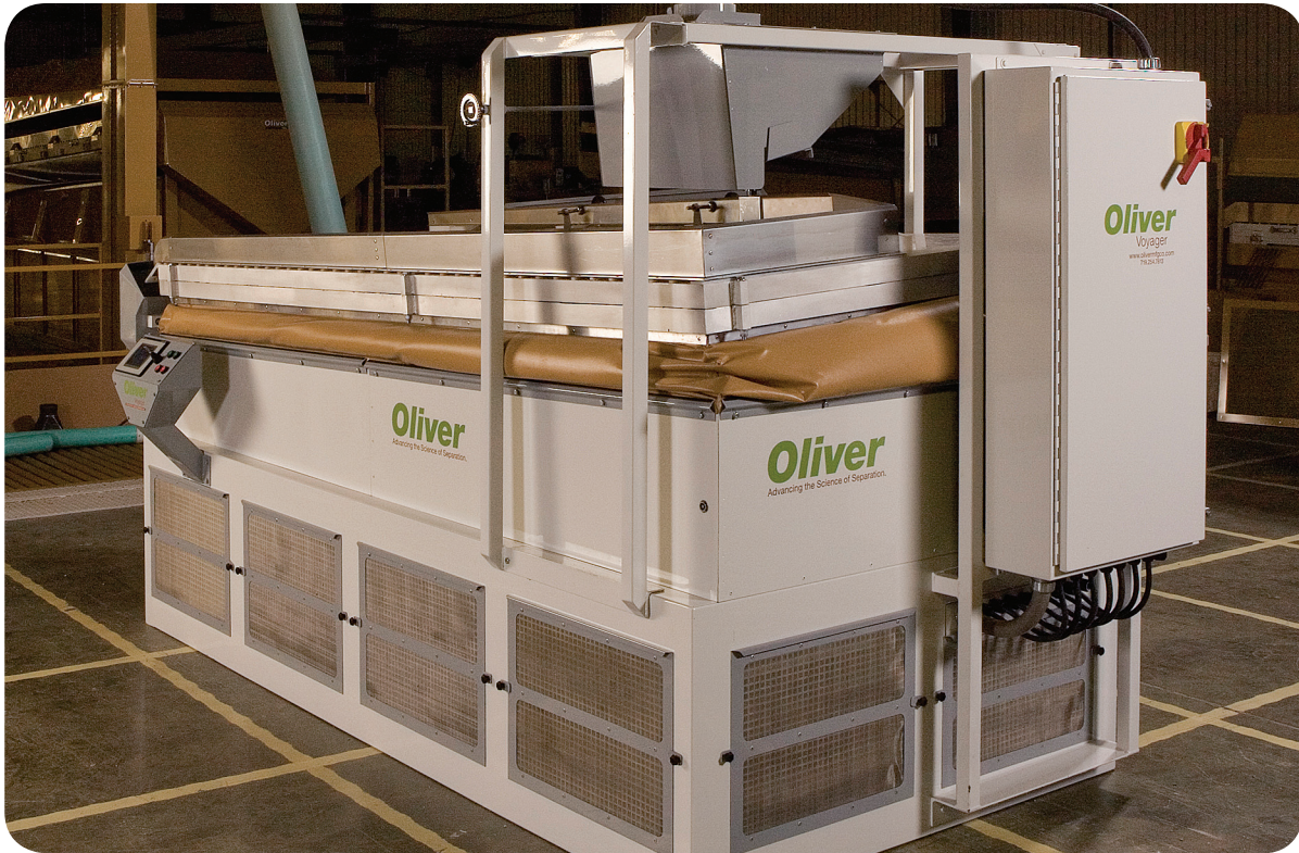
The Voyager is the first fully automated, programmable gravity separator.
